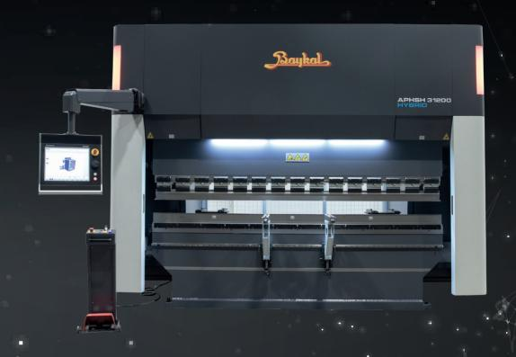
The brushless engines are directly connected to two small oil tanks. The advantage is that the cnc press brake is more precise and is not affected by temperature variation, as opposed to traditional machines.
